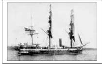
(Right above: At the outset of their career, the 'Calypso-Class' ships were apparently considered to be superior vessels. Hybrids - powered by both steam and sail - they were able to police the outer reaches of the British Empire most efficiently and economically. The rapid progress in engine technology, however, was to mean that HMS 'Calypso' and her sister-ships would soon be out-classed by newer vessels. — This Royal Navy
